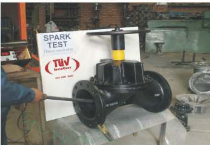
FEP Lined Diaphragm valve in Petrochemical Acid line
